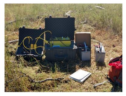
The central machine uses two electrodes to inject current, and two electrodes to measure voltage in the ground:
