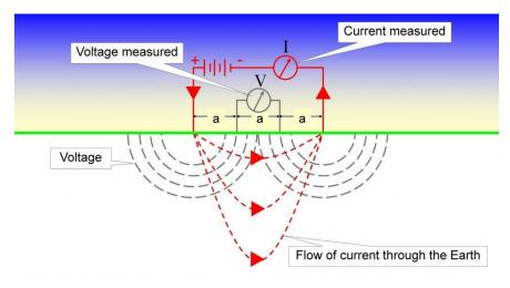
The machine automates these measurements along the profile to build up a two-dimensional cross section of the subsurface.
