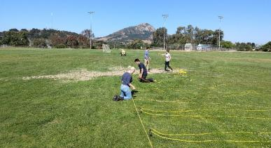
Electrodes are all connected by cables to a central unit that controls the survey.
