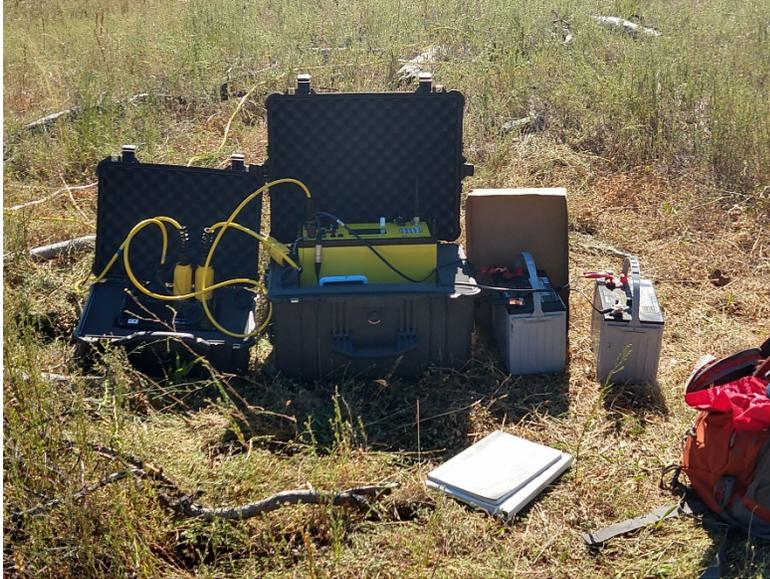
The central machine uses two electrodes to inject current, and two electrodes to measure voltage in the ground:
